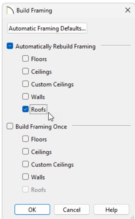
In X15 and Home Designer Pro 2024, check the **Build Roof Framing** or **Automatically Build Roof Framing** box located on the Roof panel of the **Build Framing** dialog instead, then click **OK**.
