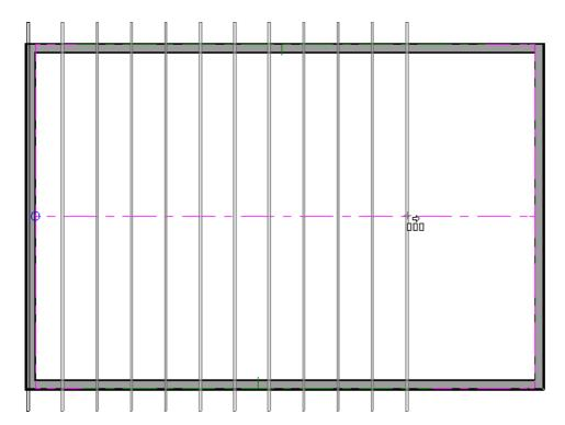
The trusses located on each end of the structure will be a full size trusses. If you wish to have end trusses instead, group select the trusses on each end, open them up to specification, check the "End Truss" and "Force Truss Rebuild" boxes, then click OK.
