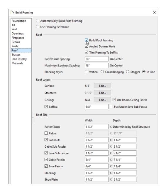
Automatic trusses, along with any other automatic framing components, such as blocking and fascia boards, will be generated.
