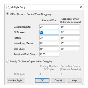
7. Hover over the main Move edit handle on the truss until you see the **Multiple Copy** cursor display, then click and drag across the structure to create copies 24" apart.
