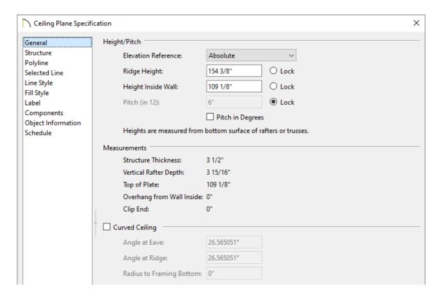
Specify the **Pitch** to match the roof that was generated in the section above. If the Pitch field is grayed out,
