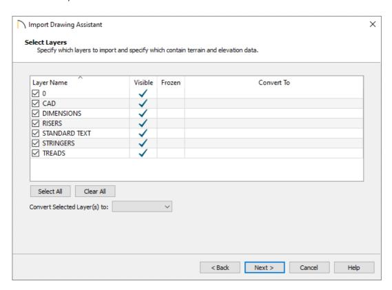
**Note:** If an imported layer is converted to Elevation Data, any points and lines on that layer are converted to Elevation Points and Lines, and any elevation data associated with them is preserved.
