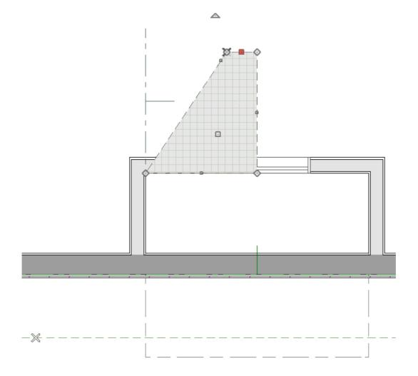
• Drag the short edge of the roof plane outward until it disappears and the roof plane becomes a triangle.
