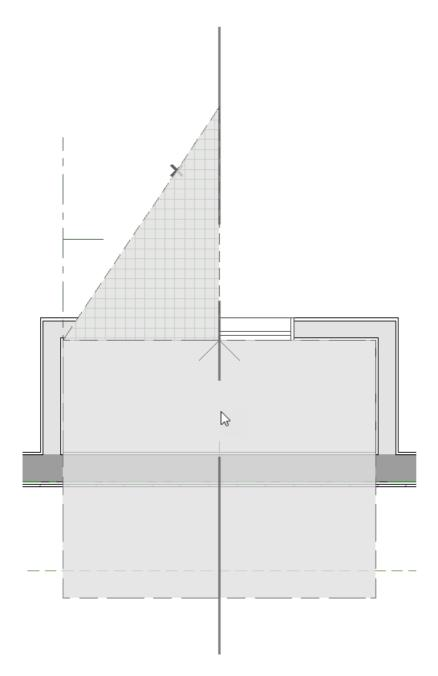
• Copy/reflect the roof plane about the fireplace to produce a roof plane that slopes in the opposite direction as the original.
