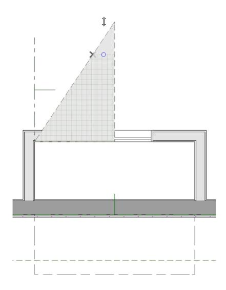
8. Use the **Copy/Paste** and tool in combination with the **Reflect About Object** edit tool to create a copy of the cricket roof plane.
