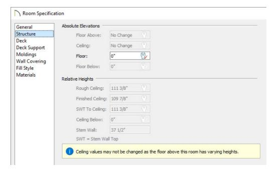
It is recommended that you setup the floor and ceiling height defaults for all of your floors to reflect the most common values for the rooms on each floor. Then, start on the lowest floor and work your way up in order to modify floor and ceiling heights for rooms that do not adhere to the specified defaults.
