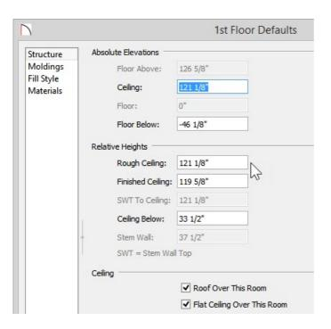
3. Select **Build> Cabinet> Soffit** and place a soffit within the area where a suspended ceiling is going to be drawn.
