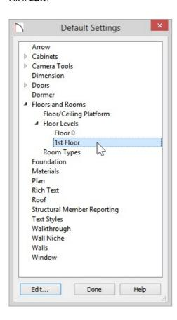
2. In the **1st Floor Defaults** dialog, on the **S**TRUCTURE panel, specify **Ceiling** as the height of the structural ceiling. In this article 121 1/8" is used. When done click **OK** to close the dialog and click **Done** to close out of Default Settings.
