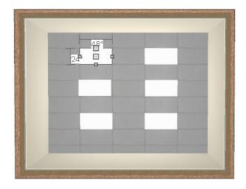
If you have trouble getting the light within the grid hold down the Ctrl/Command key on your keyboard to allow for free movement.
