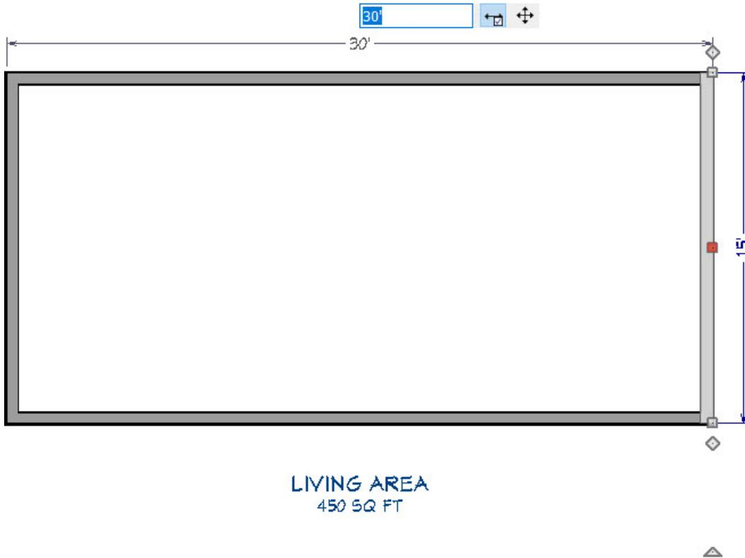
3. With the input field active, use your DISTO™ measuring device and take a measurement.
