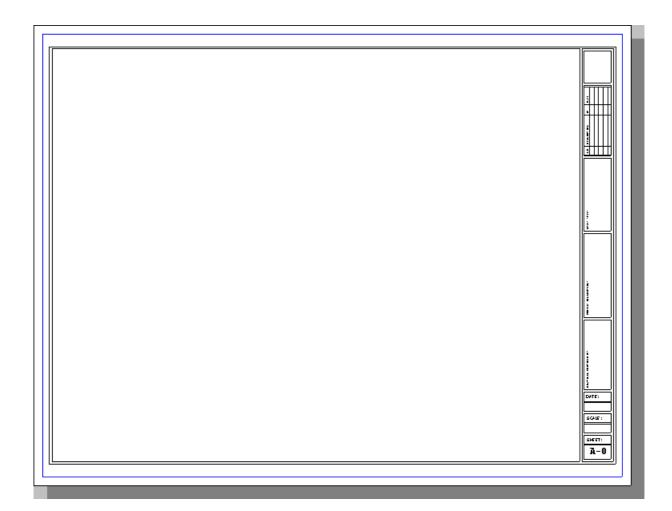
The blue border represents the printer margins that are specified in the Drawing Sheet Setup dialog. Anything located outside of the blue border will not be printed.
