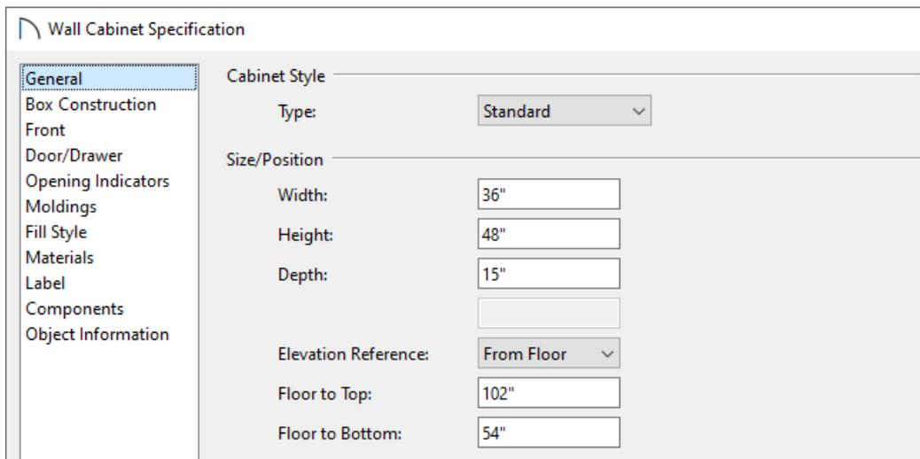
The screenshot shows the 'Wall Cabinet Specification' dialog box with the 'General' panel selected. The 'Cabinet Style' is set to 'Standard'. The 'Size/Position' section includes the following settings:
