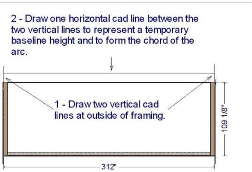
You know that the Chord of the Arc will be 26' (or 312"). You have yet to determine the roof ridgeline height and the Arc Radius for your barrel roof.
