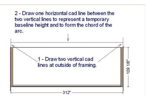
You know that the Chord of the Arc will be 26' (or 312"). You have yet to determine the roof ridgeline height and the Arc Radius for your barrel roof.
