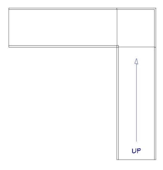
While the landing shown in this example is drawn at a right angle of 90 degrees, keep in mind that, as with stairs, we could draw these two segments at various angles and still generate a landing between them. Here are two simple examples:
