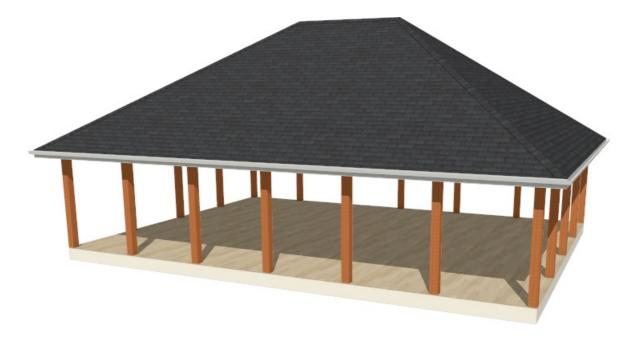
By default, the program will generate a roof plane over each exterior wall, defining a hip roof.
