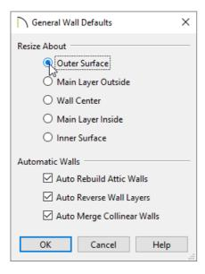
These radio buttons determine what part of a wall retains its position when its wall type or wall type definition is changed.
