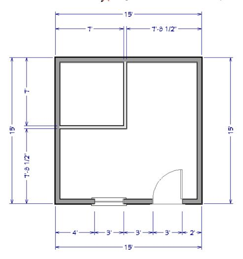
Auto exterior dimension lines locate walls as specified in the Dimension Defaults dialog.
