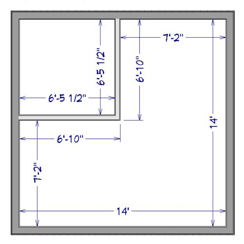
Auto room/interior dimension lines are generated inside of the rooms they measure and locate the interior surface of walls and openings.
