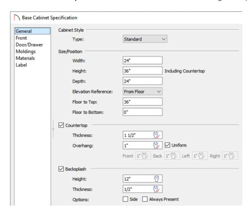
• On the General panel, check the **Backsplash** box, then set the **Height** and **Thickness** to your desired values.
