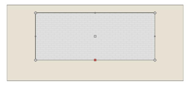
**Note:** You can use the Break Line edit tool when the backsplash is selected to place break points along a desired edge. This will provide greater flexibility for adjusting the shape of the backsplash.
