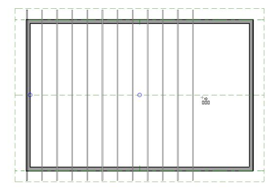
7. Next, with the **Select Objects** tool, select the trusses on either end of the structure and click the **Open Object** edit button.
