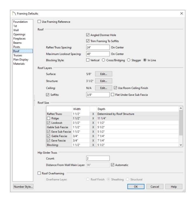
4. Once your roof framing settings are setup to your liking, click **OK**, check the appropriate **Roofs** box in the **Build Framing** dialog, then click **OK**.
