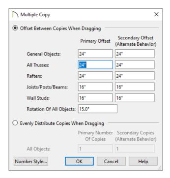
6. Hover over the main Move edit handle on the truss until you see the **Multiple Copy** discussor display, then click and drag across the structure. As you drag, new trusses will be created at regular intervals. Release the mouse button to complete the command.
