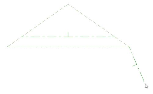
It is recommended that you examine that baseline and its roof plane to make sure that the baseline direction is correct. If it is not, you can restore the original direction by selecting **Edit> Undo** from the menu.
