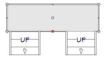
2. With the landing edge selected, click the **Add Break** — edit button, then click once between the two stair sections to break the landing's edge into two separate segments.
