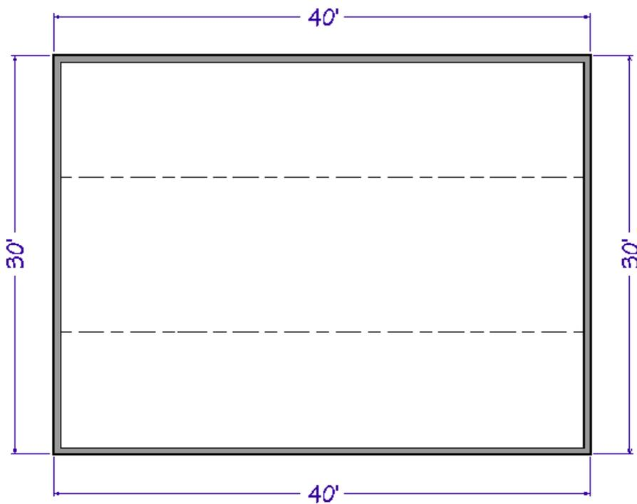
5. Select **Build> Wall> Straight Interior Wall**
