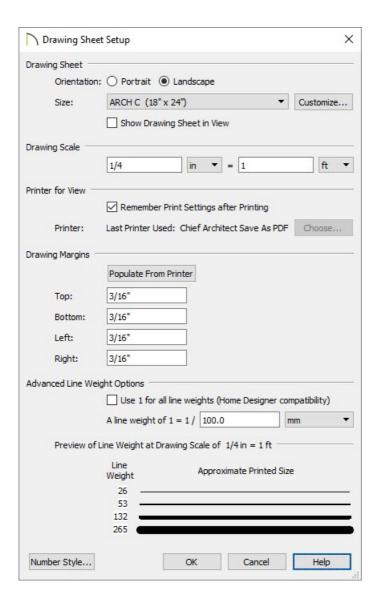
• Under Advanced Line Weight Options, make a note of the value and units listed next to **A line weight of**.
