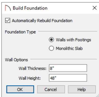
**Note:** If the foundation's Wall Height is less than 76" (1900 mm), an automatic slab floor will not be created.
