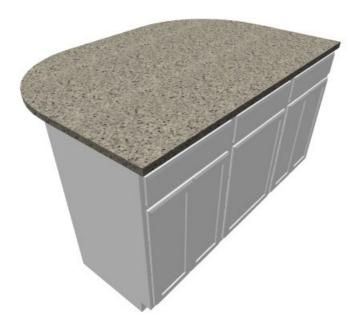
7. The cabinet can be customized further through the cabinet's depth, handles and hinges, shelf, door and drawer options in the Base Cabinet Specification dialog. The materials that make up the different components of the cabinet can also be customized within the Base Cabinet Specification dialog, under the MATERIALS panel.
