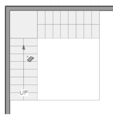
4. Click to place the stair at the desired location and the stair will be placed with a landing connecting the different stair sections.
