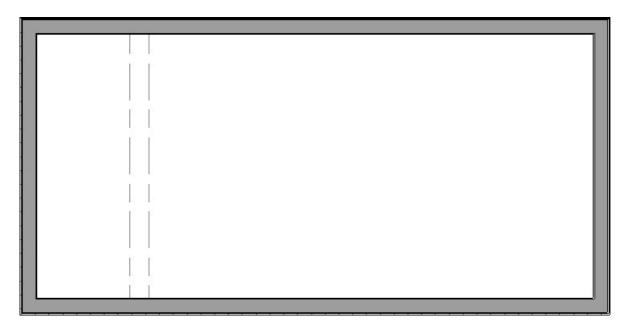
In this example, a 10' x 20' room is present and a soffit is placed spanning a distance of 109".
