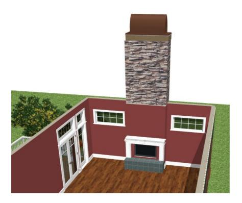
To create the appearance of a masonry chimney, you can apply a stone, block or brick material to the chase that you created using Interior Walls in the walls' specification dialogs.
