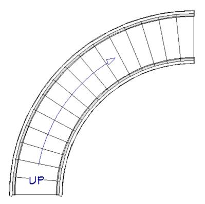
6. At this point, the curved wall segments will likely conflict with the start of the staircase, which can be verified in a camera view. When this occurs, select the curved wall segments using the **Select Objects** tool, then adjust their length so they start at the second tread of the staircase.
