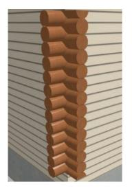
7. Repeat this process for the remaining corners of the structure, making sure that 8-13 Full and 8-13 Half corners do not share the same wall, but are always around the corner from one another.
