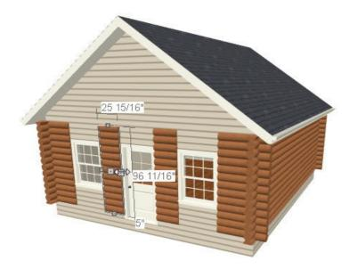
To complete the exterior, you need to fill in the areas under the door and windows, and in the gable area, which can be accomplished using individual horizontal logs.
