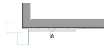
You can click anywhere in floor plan view to place it; however, if you click close to the exterior of a wall, it will automatically snap onto the wall's surface with the flat side facing inward and the log facade facing outward.
