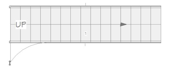
• The triangular handles that display along the long edges of the staircase are used to adjust the flare radius.
