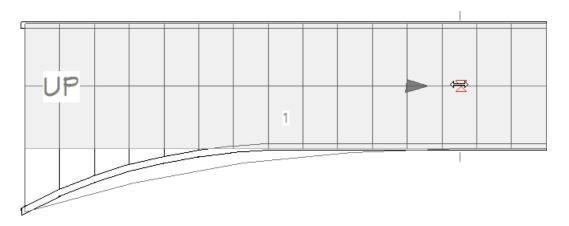
Only exposed sides of a stair section can be flared. If one side of a stair section is against a wall or wrapped, only the exposed end can be flared.
