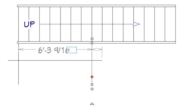
4. Select **CAD> Points> Place Point** from the menu, then click once at the point where the first and second lines meet, and once where the third line meets the edge of the staircase.
