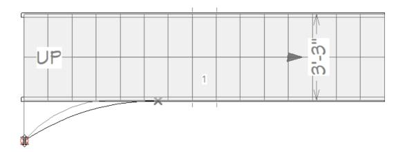
• Use the side and center edit handles closest to the flare to adjust its curve so that it closely matches that of the CAD arc.
