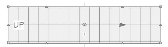
• The square handles that display at each corner of the staircase are the flare handles.
