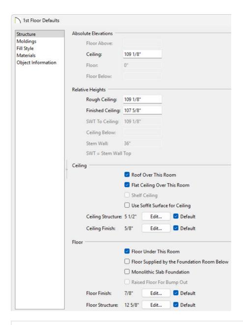
At the bottom of the Structure panel, there is a setting for Monolithic Slab Foundation. If a foundation plan is desired, do NOT check this setting. Instead, choose Monolithic Slab in the Build Foundation dialog or the Foundation Defaults prior to building the foundation. If Monolithic Slab Foundation is checked, the current Floor Structure will be replaced by a single 4" (100mm) layer of concrete with footings that can be seen in camera views only.
