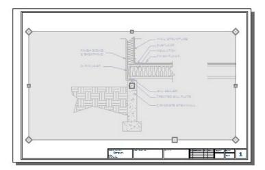
4. Using its edit handles, reduce the size of the layout view box until it only shows the details you want to see.
