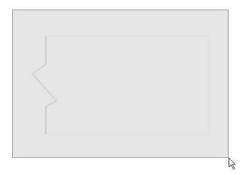
11. Use the  $\textbf{Move} \iff$  edit handle to position the break line polylines as needed in the drawing.
