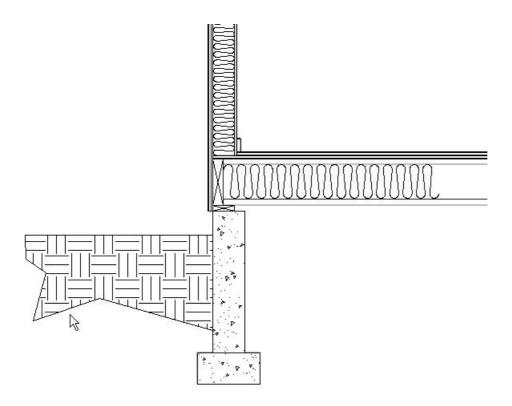
Detail drawings rarely show the entire structure. Instead, lengthy components like walls and floor platforms are truncated using a break line. If you were to draw your cross section detail by hand using the CAD tools alone, you could create a break line using a simple open polyline. Because details in Home Designer are added to a cross section of the entire structure, it may be helpful to create a closed polyline with a solid white fill to hide unneeded portions of your cross section.
