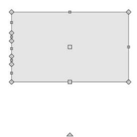
To space the breaks evenly, draw CAD lines through the polyline and position them at regular intervals using dimension lines. Then, use Object Snaps to add corner edit handles at the points where the lines intersect the polyline.
