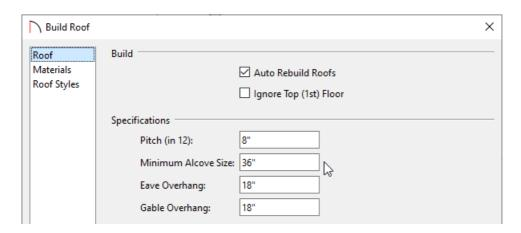
Any alcove less than the specified value is treated as though the exterior wall continues straight across. Alcoves that measure wider than this value are not roofed over; they cause a change in roof planes.
