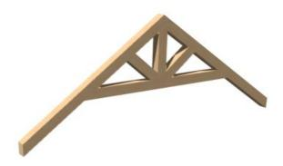
Remove the default flat ceiling and draw sloped ceiling planes to produce scissor trusses. More on creating scissor trusses can be found in the <u>Related Articles</u> section below.
