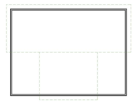
8. You can repeat this same process for the bottom roof plane, or you can simply drag the edges to match the top roof plane. To do this, use the **Select Objects** to to select the roof plane by clicking either side edge, select the **Move** the handle, and drag until it snaps to the corner of the other roof plane. Note the red indicator box marking the snap point.
