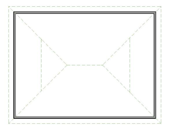
6. To connect the smaller side roof planes simply drag its edit handle until it snaps to the intersection.
