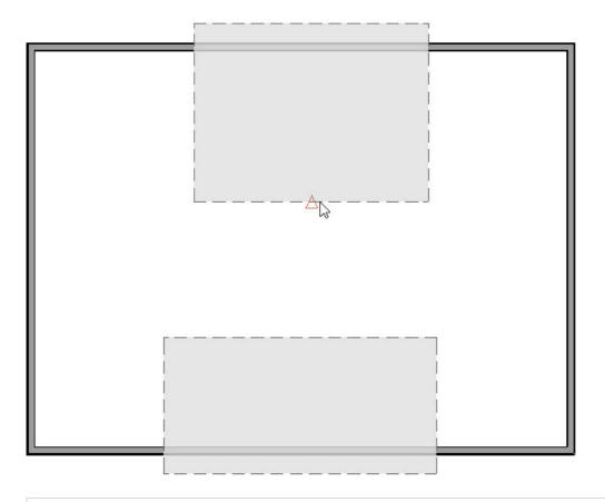
**Note:** To use the Join Roof Planes tool, you must first identify which edges of the roof planes can extend to meet at a ridge, hip, or valley. The program will try to join the two planes along the line where they intersect whenever possible.
