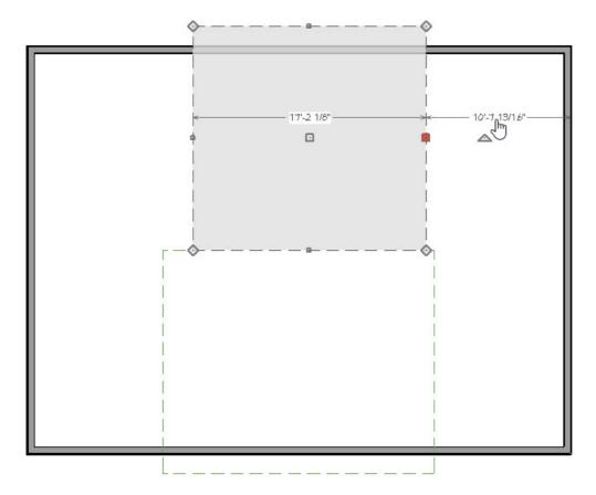
When we select the side of one of the roof planes we can see a temporary dimension line indicating its distance from the wall.
