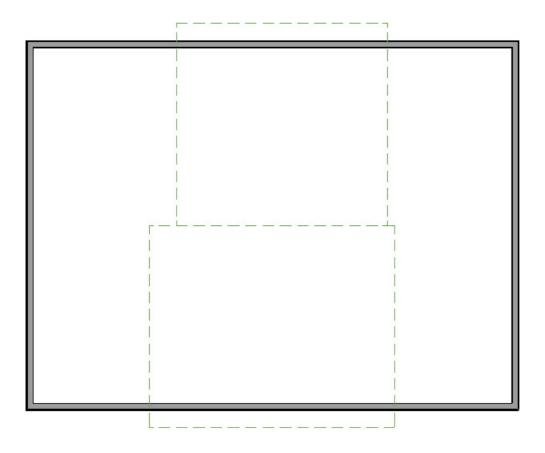
5. Now extend the sides of each roof plane so that they extend past the exterior walls.
