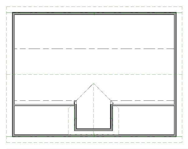
If you receive a Warning dialog stating "Hole in roof, slab, countertop, or terrain object is not completely contained.", this occurs when the roof planes are too high. This means that the joined ridgeline is generating above the main roof ridge, which can be caused by a wide dormer. Either decrease the width of the dormer being created, manually lower the roof plane baselines or lower the dormer roof pitch.
