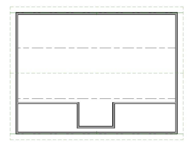
Now that the dormer walls are in place, a hole in the roof plane will be needed to allow the walls to come through in order to create the dormer.
