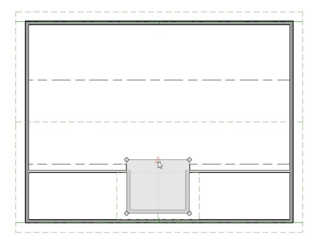
2. Using the **Select Objects** tool again, select the top edge of the left dormer roof plane, click the **Join Roof Planes** edit tool, then click on the left segment of the Roof Hole polyline.
