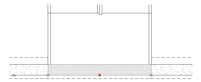
4. Using the **Select Objects** tool, select the wall section that is against the landing, click the **Open Object** edit button, and in the **Foundation Wall Specification** dialog, change the Wall Type to **Siding-6**, then click **OK**.
