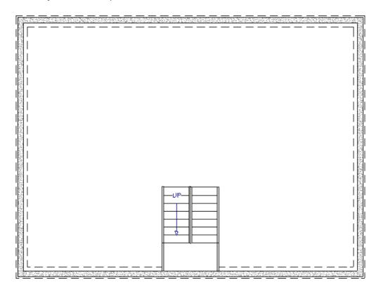
3. With the staircase in place, we are ready to modify the foundation wall for the door that will be placed later on. Select the foundation wall that the landing is against, select the **Add Break** — edit tool, then place two break points where the landing meets the foundation wall.
