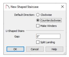
2. You will notice that a U-shaped staircase is now following your cursor. Hover the cursor along the wall that will be used for the entry, move the cursor towards the center of the structure until the landing is oriented correctly, then click to place the staircase.
