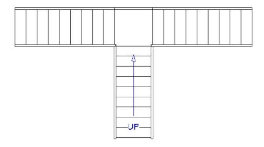
5. Finally, position the third staircase to precisely intersect with the landing.
