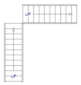
3. With the **Draw Stairs** tool still selected, click in the empty space between the two staircases. A landing will be created. At this point, two staircases in an L-shape design connect and share a landing.
