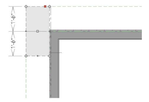
8. With the roof plane still selected, click on the corner edit handle where the ridge and outside edges meet and drag it in until it meets the corner of the wall.
