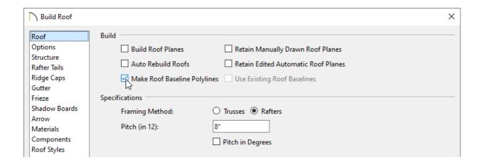
Roof Baseline Polylines display either the pitch of the roof plane bearing on each exterior wall or "(VERT)-G" when the wall has a gable above.
