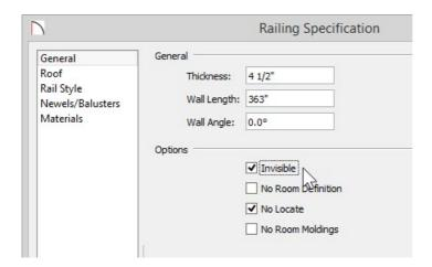
5. Notice that the three railings that make up the portico have been set to be invisible and now display as dashed lines as shown in the image below.
