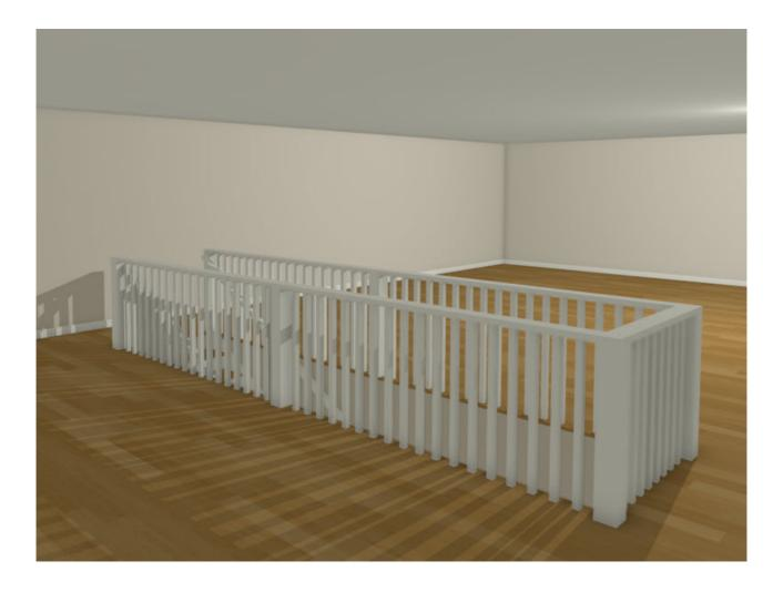
4. With the stairwell generated, you can select and edit the railings encompassing the stairwell room to change them to solid, adjust their height, materials, or make any other desired changes, as necessary.
