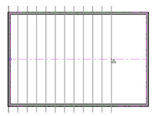
The trusses located on each end of the structure will be full size trusses. If you wish to have end trusses instead, select the trusses on each end, open them up to specification, check the "End Truss" and "Force Truss Rebuild" boxes, then click OK.
