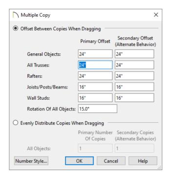
5. Hover over the main Move edit handle on the truss until you see the **Multiple Copy** cursor display, then click and drag across the structure to create copies 24" apart.
